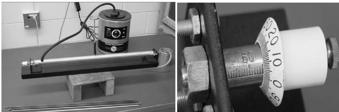
Figure on the left: linear expansion apparatus. Here, the rods are placed inside the silver jacket and the whole assembly is placed on the black base. (Photo credit: IISER Pune, ( http://www.iiserpune.ac.in/~bhasbapat/phy221_files/lab1.pdf ) (As on 31st July 2021))
